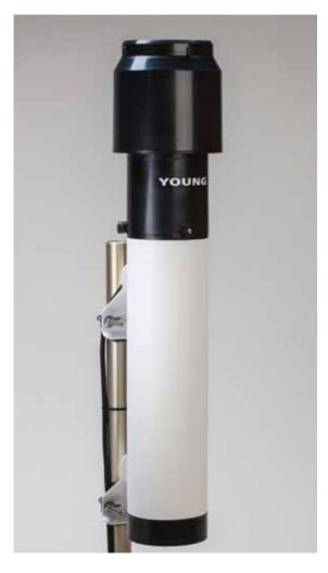
When the column level reaches a maximum of 250 mm (50 mm of precipitation), the chamber automatically empties and the process repeats. Total precipitation can be tracked by a datalogger or recorder.
