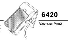
The sensing grid is a gold-plated etched circuit on an epoxy-glass substrate; the excitation and sense circuits are encapsulated in black epoxy. The included mounting bracket holds the sensor at a 45° angle to simulate a typical leaf position and to permit runoff of excess moisture; it may be mounted on a vertical post, pipe, or stake, or on the Sensor Mounting Arm.
