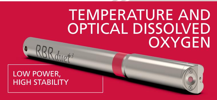
The RBRduet<sup>3</sup> T.ODO is a small temperature and optical dissolved oxygen instrument with low power consumption and high stability. The |fast variant has a time constant of only 1s and is well suited for profiling applications. The |slow version has a protective layer to facilitate automated cleaning by a wiper, which keeps it biofouling-free during long-term moored deployments.
